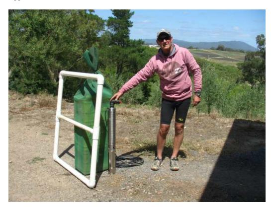
Richard is displaying the submersible pump cylinder (25kg) with its power input cable, laying next to the filter box. We made the filter box out of 3 soft-drink cases tied together with cable ties and wrapped in shade cloth. The filter box is downside up in this photo. The float made out of hard poly-pipe is nearest camera.
