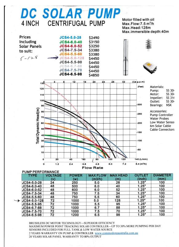
Annotations show which pump we installed at La Grue Olives -- JCS4-5.0 - 128.
